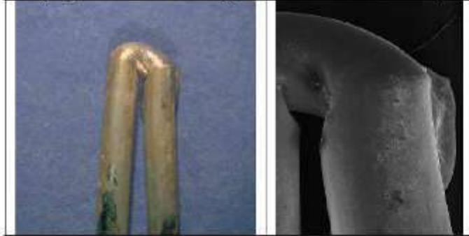
**Figure 3 SEM images of arc bead interior.**
