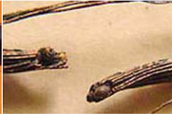
Arc severing & subsequent beading\*
