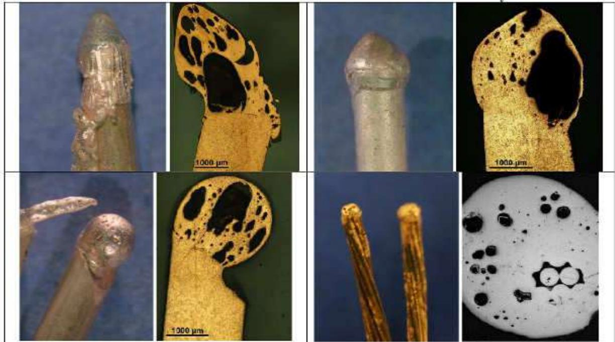
**Figure 6 Stereomicroscope and optical micrographs of fire melting damage to solid and stranded conductors created in the laboratory.**
