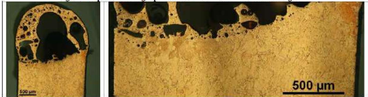
E.C. Buc, D. Reiter, J. Battley, T.B. Sing, T.M. Sing, METHOD TO CHARACTERIZE DAMAGE TO CONDUCTORS FROM FIRE SCENES
